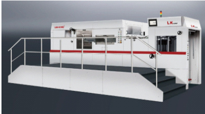
LK106MF – Automatic Die cutting machine, format 106 x 78 cm, with hot foil stamping
