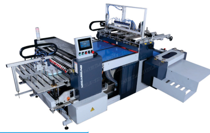
CASEMAKER ULTRA – Automatic, feeding and folding on 4 sides
