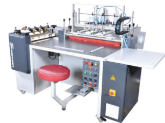
CASEMAKER ACTIVE PLUS - Automatic, arming and lining hardcover, 2-sided
