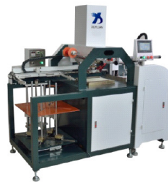
XY-TY2016 – Hot Stamper with automatic sheet feeder
